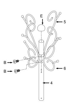
4/ Attach top unit to base unit by using screw (B) as shown.
