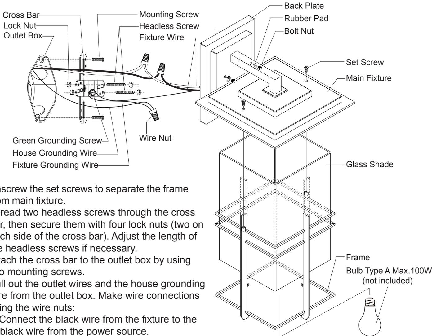
1. Unscrew the set screws to separate the frame from main fixture.
