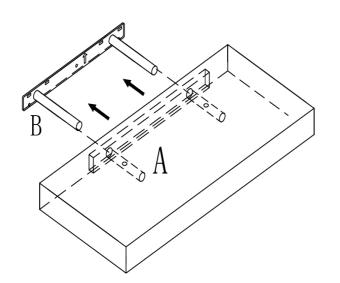
Slide shelf (A) onto the mounting bracket (B) by aligning the two holes on shelf (A) to the poles on bracket (B), making sure the two small holes are pointing down on the bottom of shelf (A).
