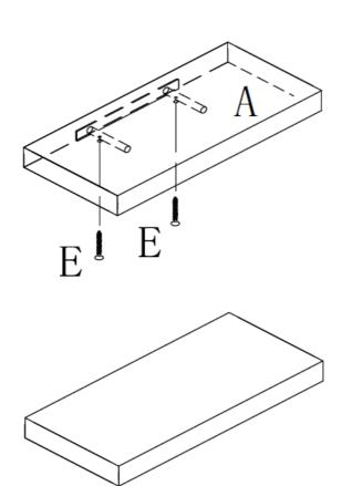
Insert the two long screws (E) with a screwdriver to secure shelf (A) to bracket (B).
