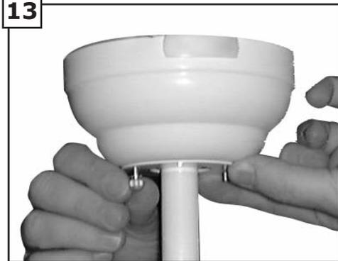
13 Next lift the cover ring and install knurled nuts as shown. Tighten the knurled nuts securely. The canopy should adjust for any irregularity in the ceiling or Outlet box.
