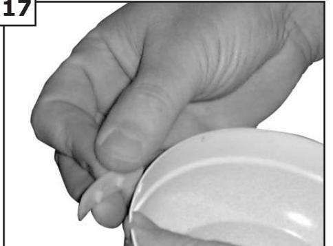
17 Remove side covers from canopy exposing 4 holes. 2 closed holes and 2 open "L" shape holes.
