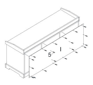
Attach back panel (I) to assembled unit with screws (5).
