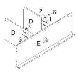
Insert cam locks (2) into holes on middle panel (D).
