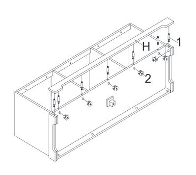
Insert cam locks (2) into holes on assembled unit as shown.
