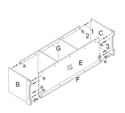
Insert cam locks (2) into holes on bottom panel (E), rear cross panel (F), and front cross panel (G).
