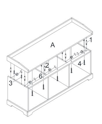
Insert cam locks (2) into holes on assembled unit as shown.
