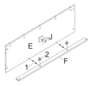
Insert cam locks (2) into holes on back cross Panel (F).
