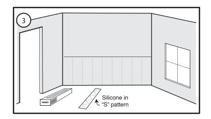
Adhere the plank to the wall leaving a 3/16" gap (A) from the corners of the wall and a 1" gap (B) at bottom. Drive brad nails  $\frac{1}{2}$ " from the top and bottom of each plank to secure to wall. Place nails where the trim will cover.
