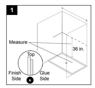
Check the measurements, and then place masking tape (not included) over the area where the saw (not included) will contact the finished side of the lower back panel (A). Cut the lower back panel (A), and make any final adjustments to the cuts with a sanding block (not included).
