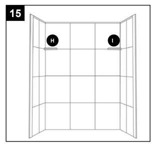
Once installation is complete, seal all the joints with silicone adhesive/sealant (K). Note: Clean all joints with denatured alcohol before applying a uniform bead of silicone adhesive to the joints.
