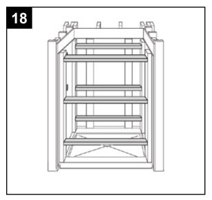
Insert small blocks (not included) between the rear panel braces and the back panel braces. These will apply pressure to the back panel to hold it in place. Remove the braces after 24 hours.
