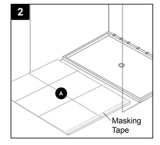
3. If needed, place 1/16 in. thick shims (not included) at the base of the lower back panel's (A) installation site. Trial fit the lower back panel (A) on the shims and use a sanding block if any fine adjustments are needed. Remove lower back panel (A) from wall and clean the back of the lower back panel (A), the wall board and any other area that will be in contact with the silicone (K) with denatured alcohol and a clean rag (both not included).
