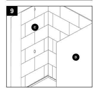
10. If needed, place 1/16 in. thick shims at the base of the left side panel (C) and right side panel (D) installation site. Trial fit the left side panel (C) and right side panel (D) on the shims and use a sanding block if any fine adjustments are needed. Clean the back of the left side panel (C) and right side panel (D), the wall board and any other area that will be in contact with the silicone adhesive (K) with denatured alcohol and a clean rag (not included).
