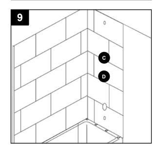
10. If needed, place 1/16 in. thick shims at the base of the left side panel (C) and right side panel (D) installation site. Trial fit the left side panel (C) and right side panel (D) on the shims and use a sanding block if any fine adjustments are needed. Clean the back of the left side panel (C) and right side panel (D), the wall board and any other area that will be in contact with the silicone adhesive (L) with denatured alcohol and a clean rag (not included).
