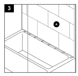
4. Cut eleven 4-in. strips of installation tape (N) and place them on lower back panel (A) where indicated in figure 4. Apply silicone adhesive (L) in 3/4 in. diameter dots every 6-7 in. apart over the surface of the reinforcement strips on the back of lower back panel (A). Place the lower back panel (A) in place and press firmly.
