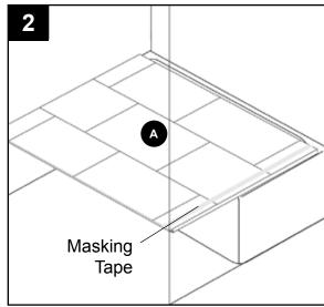
3. If needed, place 1/16 in. thick shims (not included) at the base of the lower back panel's (A) installation site. Trial fit the lower back panel (A) on the shims and use a sanding block if any fine adjustments are needed. Remove lower back panel (A) from wall and clean the back of the lower back panel (A), the wall board and any other area that will be in contact with the silicone (L) with denatured alcohol and a clean rag (both not included).
