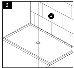
4. Cut twelve 4-in. strips of installation tape (M) and place them on lower back panel (A) where indicated in figure 4. Apply silicone adhesive (K) in 3/4 in. diameter dots every 6-7 in. apart over the surface of the reinforcement strips on the back of lower back panel (A). Place the lower back panel in place and press firmly.
