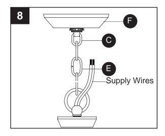
9. Unthread the canopy lock ring (D) and slide canopy lock ring (D) and ceiling canopy (F) down the fixture chain (E). Push all slack fixture wire through canopy chain loop (C) into outlet box. Trim excess fixture wire, leaving a minimum of 6 in. hanging out of the outlet box. Refer to the next step to connect the wires. Then re-attach the ceiling canopy (F) as shown in step 6.
