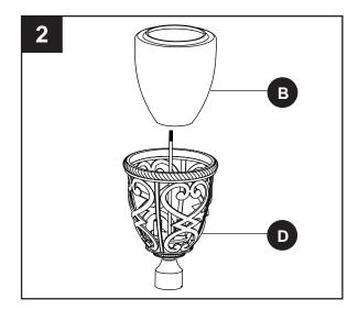
3. Carefully fit the post fitter on the fixture body (D) over the end of the post (not supplied), making sure the post fitter is fully seated. Mark the drill point for the 3 mounting screws using 3 mounting holes as reference. After marking hole locations, remove fixture from post and drill 1/16 in. pilot holes for screws.
