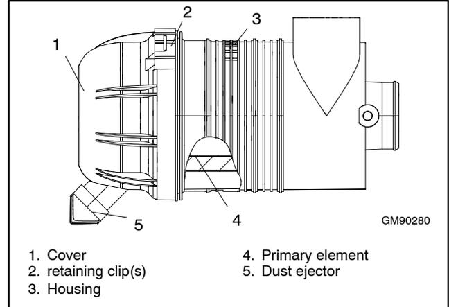
**Figure 8** Air Cleaner; 24RCL, 30RCLH, 60RCL
