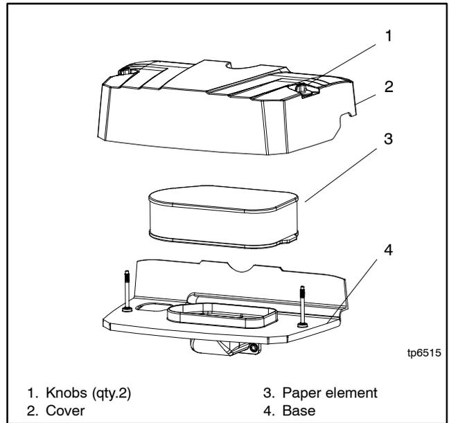
**Figure 6** Air Cleaner; 17/18RES(L), 20RES(A)(AL)(B)(L)
