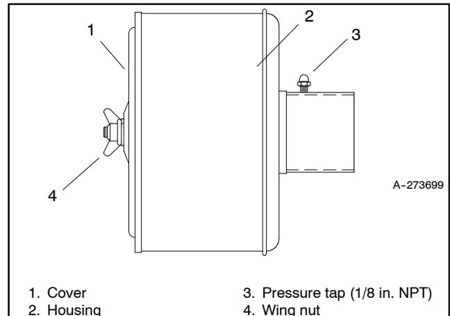
**Figure 9** Air Cleaner; 38RCL, 48RCL
