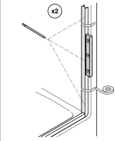
**6** Drill 5/16" holes and insert the anchors.
