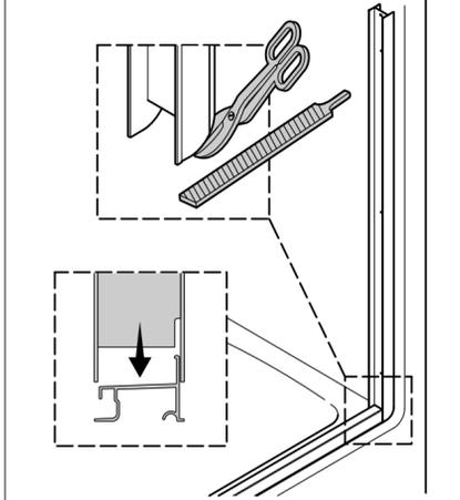
**5** Plumb both wall jambs. Mark the screw holes.
