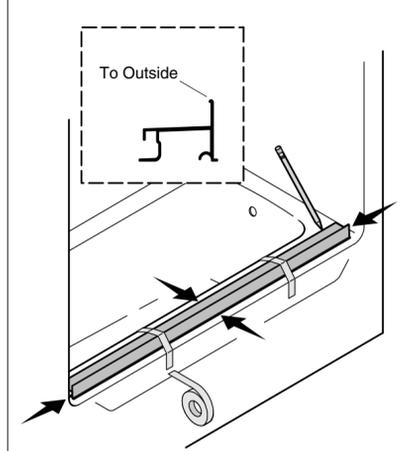
**4** Position the wall jambs over the bottom track. Snip/file bottom edges for a snug fit.
