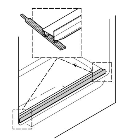
**3** Center the bottom track on the ledge with the leg to the outside. Tape in place and mark position.
