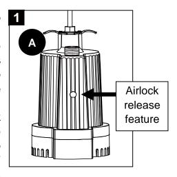
CAUTION: This valve is for anti-airlock purposes. Leakage of air or water is NORMAL. DO NOT REMOVE or PLUG THIS VALVE!
