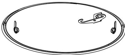
Recessed Housing Typical Spring Retaining Bracket
