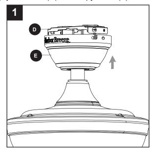
Secure the canopy (E) with the mounting bracket screws (U) previously removed (Step 4, page 8).
