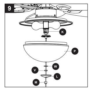
10. Attach the pull chain extensions (EE) or custom pull chain extensions (not included) to the fan and light pull chains.
