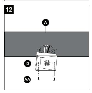
13. Once the lantern post (A) is completely assembled, secure the lantern post (A) into the hole with concrete (not included). Note: Ensure the bottom of the lantern post (A) is embedded in the gravel and is level before pouring the concrete up to just below the inlet hole. DO NOT pour concrete up to the ground level.
