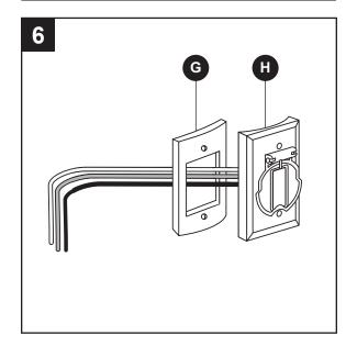
7. Route the wires from the convenience outlet (H) through the empty hole and out the hole with the supply and lantern wires.
