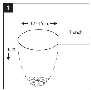
2. Run the electrical cable (not included) through the trench from the power supply to the hole created for the lantern post (A).
