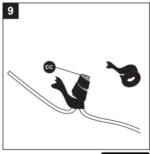
10. Gently push the wires and wire connectors (CC) into the pole.
