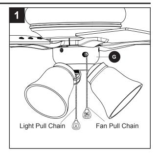
Using a ceiling fan will allow you to raise your thermostat setting in summer and lower your thermostat setting in winter without feeling a difference in your comfort. Note: Wait for the fan to stop before moving the reverse switch located on the light kit (G).
