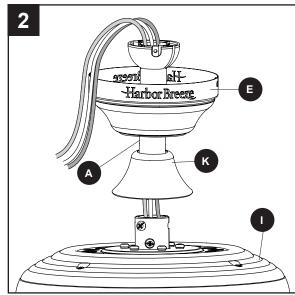
3. Slide the downrod (A) into the yoke of the motor assembly (I), align the holes, then re-install the downrod pin (B) and downrod clip (C). Secure with set screws (P) and slide the yoke cover (K) down until it rests on top of the motor assembly (I).
