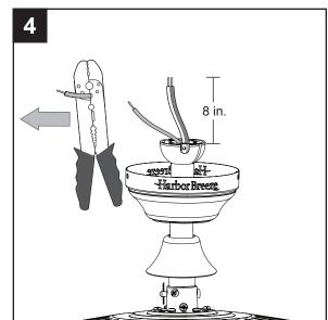
5. If you decided to cut back the lead wire in Step 4, strip 1/2 in. of insulation from the end of the white wire. Twist the stripped ends of each strand of wire within the insulation with pliers (not included). Repeat this step for black and blue wires.
