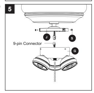
6. Assemble the light kit (G) to the fitter plate (J) using the previously removed fitter plate screws (S).
