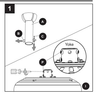
2. Insert the downrod (A) through the canopy (E) and yoke cover (K). Feed the wires from the motor assembly (I) through the downrod (A).
