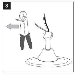
If you decided to cut back the lead wire in Step 8, strip 1/2 in. of insulation from the end of the white wire. Twist the stripped ends of each strand of wire within the insulation with pliers (not included). Repeat the step for black and green wires.
