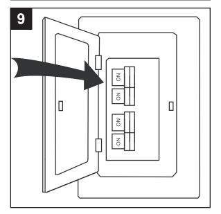
9. Turn on the circuit breakers and the wall switch to the fan supply lead lines.
