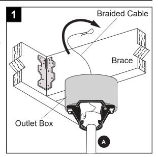
2. Install secondary support screw (FF), secondary spring washer (HH) and support washer (GG) partly into the side of the brace installed in the ceiling. Then loop the braided cable up and over the ceiling brace and place the open loop of the braided cable around the secondary support screw (FF).
