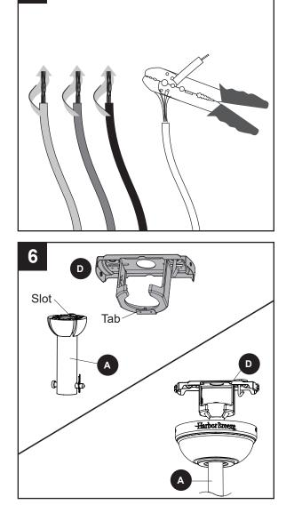
Install the ball end of the downrod (A) into the opening of mounting bracket (D). Align one of the four slots in the ball with the tab in the mounting bracket (D).
