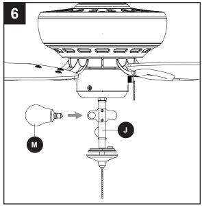
Remove the preassembled finial (L), finial cap (K), hex nut (T) and rubber washer (U) from the light kit (J). Lift the glass bowl (N) onto the threaded rod at the bottom of the light kit (J).
