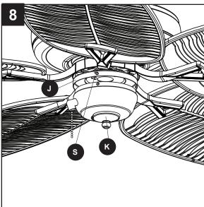
9. Attach the pull chain extension (BB) or custom pull chain extension (not included) to the fan pull chain.
