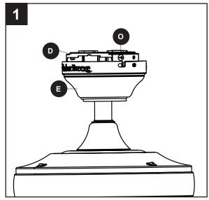
2. Secure the canopy (E) with the mounting bracket screws (O) previously removed (Step 4, page 8). Tighten all mounting bracket screws (O) securely.
