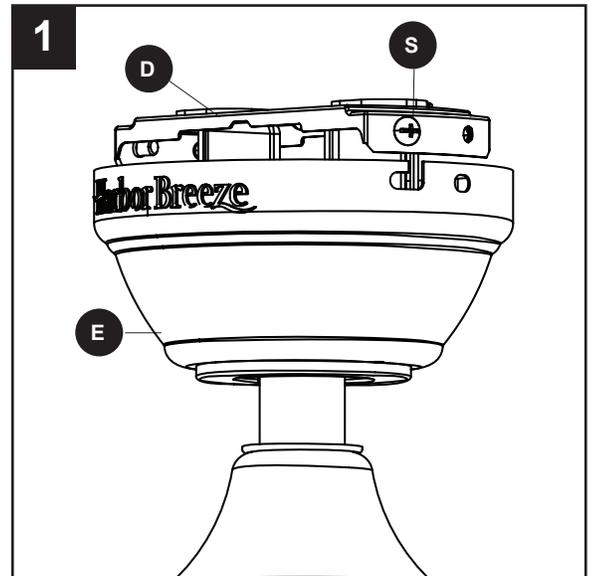
2. Secure the canopy (E) with the mounting bracket screws (S) previously removed (Step 4, page 8). Tighten all mounting bracket screws (S) securely.
