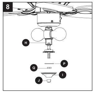
9. Lift the glass shade (K) onto the threaded rod at the bottom of the light kit (H). Re-install large washer (P) and secure with hex nut (Q). Lift the finial cap (I) onto the threaded rod and then screw the finial (J) onto the threaded rod to secure.
