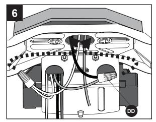
6. Turn the spliced/taped wires upward and gently push the wires and wire connectors (DD) into the outlet box.
