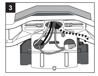
Temporarily lift the motor housing (A) to the upper mounting bracket (B) to determine which two motor housing screws (T) in the sides of the upper mounting bracket (B) align with the slotted holes in the top edge of the motor housing (A). Partially loosen the two motor housing screws (T) that align with the slotted holes. Remove the other two motor housing screws (T) from the upper mounting bracket (B).
