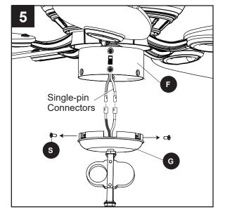
6. Align the notch in the switch housing cap (G) with the reverse switch located on switch housing (F). Then assemble the switch housing cap (G) with light kit (H) to the switch housing (F) using the previously removed switch housing screws (S).
