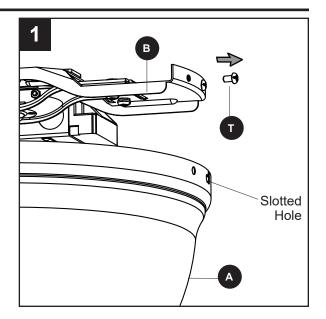
Slide the motor housing (A) over the motor (E), aligning the slotted holes in the motor housing (A) with the loosened motor housing screws (T) in the upper mounting bracket (B). Twist the motor housing (A) to lock. Then re-insert the two previously removed motor housing screws (T) and securely tighten all screws.
