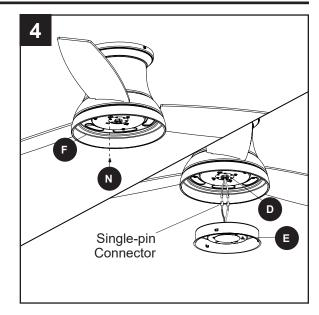
5. Align the switch housing (E) over the loosened switch housing screws (N) preassembled on the switch housing (E), then place the keyholes of the switch housing (E) onto the switch housing screws (N) and rotate the switch housing (E) clockwise. Secure the switch housing (E) with the previously removed switch housing screw (N). Tighten all three switch housing screws (N).
