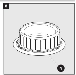
9. Insert the pop-up body (Q) into the sink and screw the flange (N) onto the pop-up body (Q). Ensure the pivot hole is facing the back of the sink. Tighten the nut (P) and remove the pivot nut (R).
