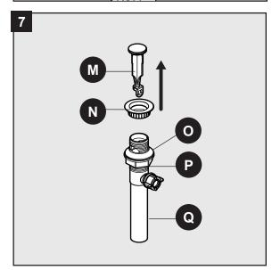
**8.** Apply silicone sealant (not included) to the underside of the flange (N).
