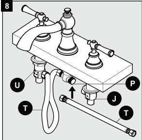
**9.** Connect a 1/2 in. IPS faucet connector (not included) to the water supplies underneath the sink using wrenches (not included).
