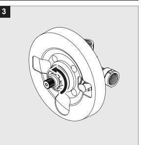
**4.** Reinstall the red limit stop ring (Q) and readjust the teeth engagement position so that the stem cannot move beyond the adjusted point.
