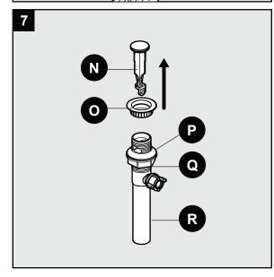
**8.** Apply silicone sealant (not included) to the underside of the flange (O).
