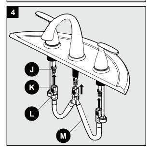
Connect a 1/2 in. IPS faucet connector or coupling nuts (not included) with 3/8 in. O.D. ball-nose risers (not included) to the water supplies underneath the sink using wrenches (not included).
