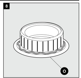
9. Insert the pop-up body (R) into the sink and screw the flange (O) onto the pop-up body (R). Ensure the pivot hole is facing the back of the sink. Tighten the nut (Q) and remove the pivot nut (S).
