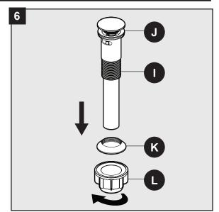
7. Insert the pop-up body (I) into the sink. Ensure that the top gasket (J) rests securely between the top of the sink and the top of the pop up body (I).
