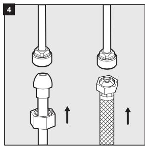
**5.** Before tightening the faucet connector to the water supply, apply a second wrench to the supply tube fitting. This will prevent the supply tube from moving or twisting when tightening the faucet connector. Do not overtighten.
