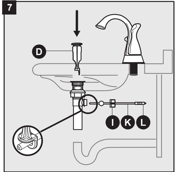
8. Re-attach the lift rod strap (J) to the horizontal rod (K) using the clip (L).
