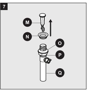
8. Apply silicone sealant (not included) to the underside of the flange (N).
