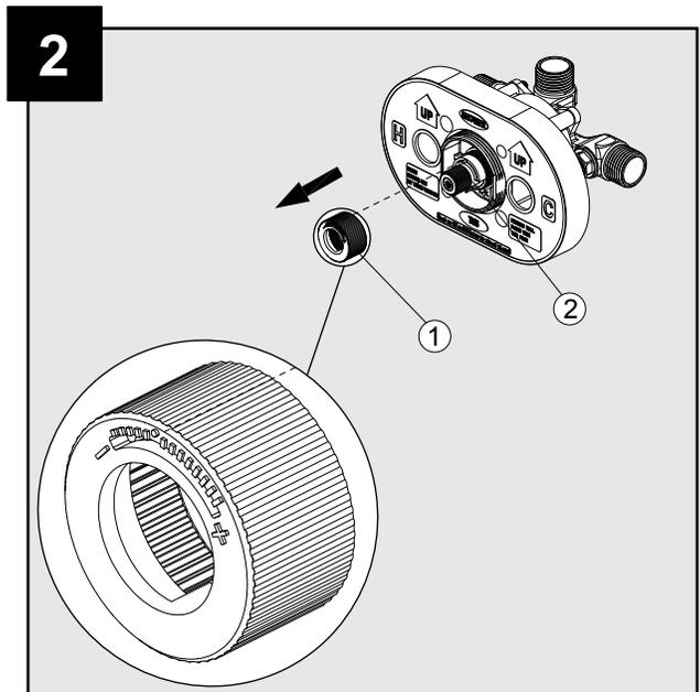
3. To adjust for the desired maximum water temperature:
