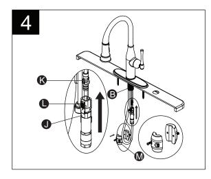
Connect 1/2 in. IPS faucet connector or coupling nuts (not included) with 3/8 in. O.D.ball-nose risers (not included) to water supplies using wrenches (not included).
