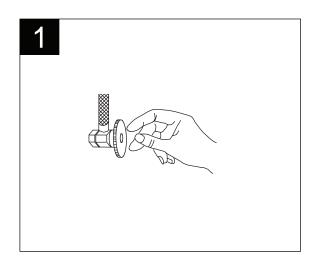
2. For single hole installation, refer to diagram 2A. Place flange (I) on the sink (not included).
