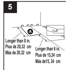
6. Angle the second plank (A) of the second row slightly upward, pushing it forward and interlocking the tongue side of the plank (A). Slide the plank (A) as necessary to the LEFT to align the edges of the plank (A) to the end of the first plank (A) of the second row.
