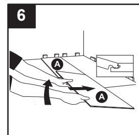
7. Once the ends align, carefully push the second plank (A) of the second row down until its tongue locks with the groove on the first plank (A) of the second row. **Note:** A slight tap with a tapping block (not included) may be necessary to complete interlock.
