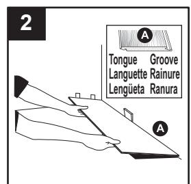
3. Align the next plank (A) over the end of the first plank (A) so the joint on the first plank (A) is tight when the second plank (A) lays flat. **Note:** Some adjustment of the planks (A) might be necessary to ensure a secure fit.
