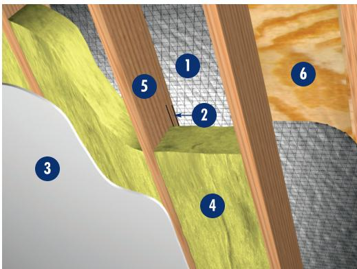
Southern Zone of the USA -With Reflectix® Above the Mass Insulation • R-6.0 Summer & R-2.0 Winter or a Radiant Barrier - Blocks 96% Radiant Heat
