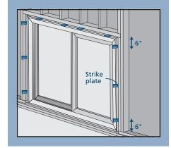
shims so that strike plate/head bracket screws will penetrate shims. 8. Inspect the patio door for square, level, and plumb. Test for proper operation (remove and reinstall if necessary).
