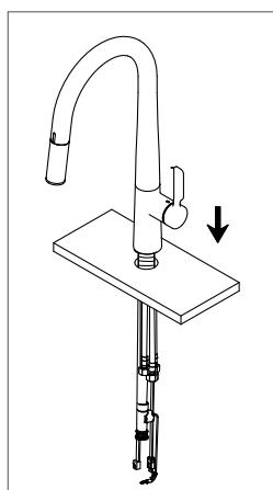
3. From underneath the sink, install the mounting hardware onto the valve shank. Be sure to thread all the hoses and cables through the washers and locknut.
