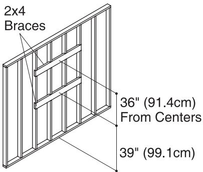
*Notch studs 1-1/2" (3.8cm) to provide support for braces*
