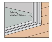
Flush fin windows must be installed onto a surface with at least a 3/8" wide exterior face. This face must be flush with or protrude past the exterior wall surface.
