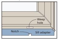
3. If the sill adapter covers weep holes, notch for proper drainage.
