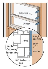
**NOTE:** On some double-hung operating units only, jamb adjuster hardware is mounted in the middle installation holes to allow for some jamb adjustment. Install jamb adjuster screws until captured (first 'click'), the screw may then be screwed in or out to adjust the jamb as needed.
