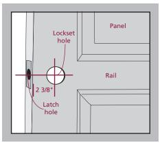
instructions and template, drill for lockset. Generally, a 2 1/8" diameter hole is needed for the lockset. Drill a 1" latch hole through the edge of the slab into the center of the lock hole to accommodate the latch for the lock. Some latches have a radius (rounded corners) or rectangular face plate that will require the slab edge to be chiseled for fit. Drill pilot holes for attachment screws. Other latches are round (contractor drive-in) and can be tapped into place with a hammer.
