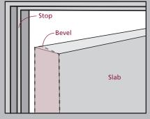
the slab face that rests against the stop becomes slightly narrower than the opposite face.
