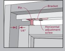
adjustments are necessary, door panels should be folded, in some cases removed, to gain access to the adjustment screws.
