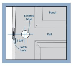
lockset. Generally, a 2-1/8" diameter hole is needed for the lockset. Drill a 1" latch hole through the edge of the slab into the center of the lock hole to accommodate the latch for the lock. Some latches have a radius (rounded corners) or rectangular face plate that will require the slab edge to be chiseled for fit. Drill pilot holes for attachment screws. Other latches are round (contractor drive-in) and can be tapped into place with a hammer.
