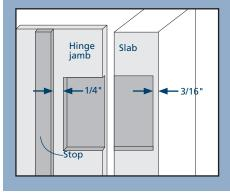
7. Using the hinge as a template, mark screw hole locations and drill pilot holes for all screws. If possible, it may be easier to remove the hinge pin to separate the hinge leaves. Use a hammer and a punch to drive the pin from the open end. Install the hinge leaves separately on the jambs and slab (we recommend using a hand screwdriver when installing screws into the slab to prevent stripping). Then, hang the slab in the frame by aligning the hinge leaves and re-install the hinge pins.
