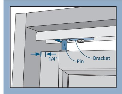
Two and four panel assemblies should have 1/4" clearance between the pivot doors and each jamb. Four panel assemblies should be snug at the middle.
