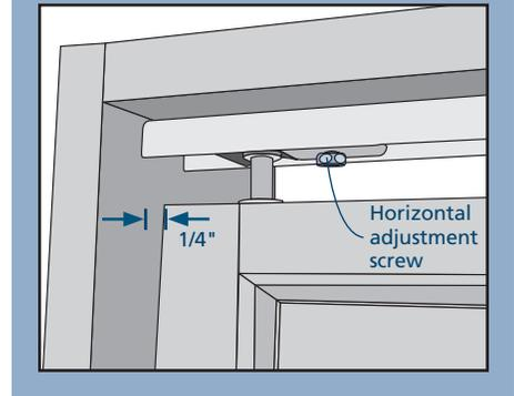
9. Loosen the screw on the snagger and close doors. Move the snagger until it contacts the guide pin. Open doors and move the snagger an additional 1/8" toward doors and tighten screw. Doors should slightly "snap" shut, but reopen easily with a tug on the knob.
