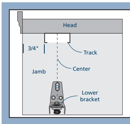
Fasten to the jamb with a 1-1/4" flat head screw through the middle of the top slotted hole.
