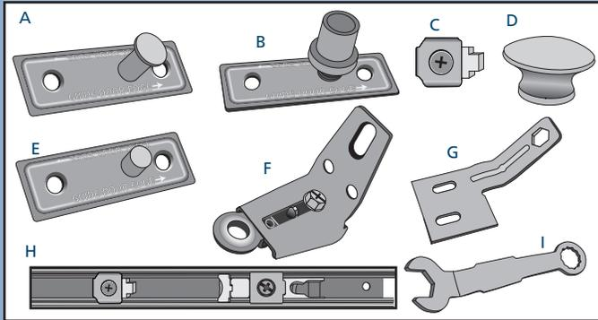
1. Position the guide, upper pivot pin and lower pivot pin on the door assembly in the locations and orientations shown.
