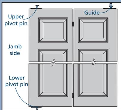
2. Measure in 5/8" from the end of each panel and center each pin on the panel.
