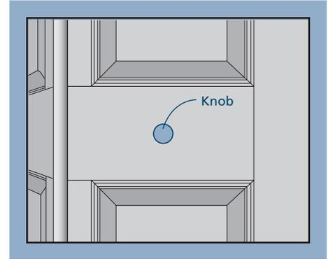
**Note!** Unless drilling the knob attachment hole close to an edge on a hollow core door, it will likely be in a hollow part of the door. This does not cause problems and the door material is sufficiently strong if the screw is snug but not over tightened.
