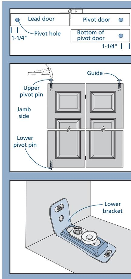
5. Place the upper pivot pin into the hole in the top pivot bracket and the guide pin into the track. Lift the assembly and place the lower pivot pin into the lower bracket. If installing a four door system, repeat for the other assembly. Check positioning and operation.
