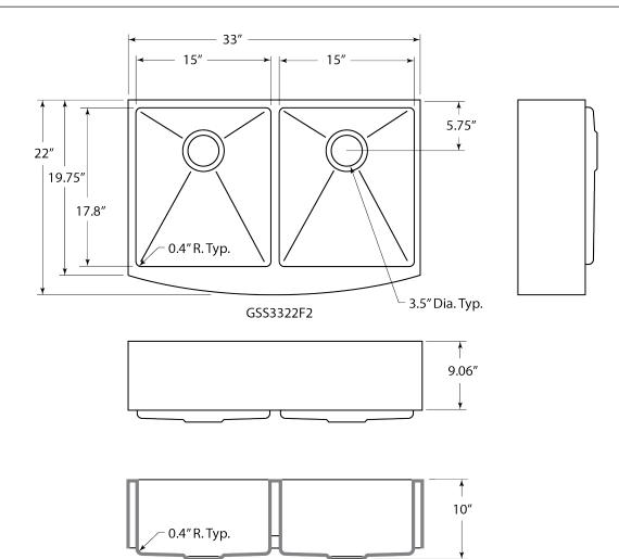
This sink is intended only for under-counter installations of solid-surface composite or natural stone countertops. It is highly recommended that this product be installed by professionals.
