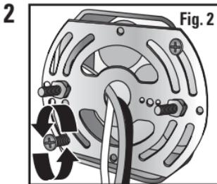
Pull the existing supply wires through the center hole of the mounting bracket. Using your old electrical box screws, secure the mounting bracket to the electrical box, make sure the protruding machine screws are parallel to the floor (Fig. 2). You may need to use the slots to mount the universal bracket so the machine screws are parallel to the floor. This will allow for leveling of the fixture.
