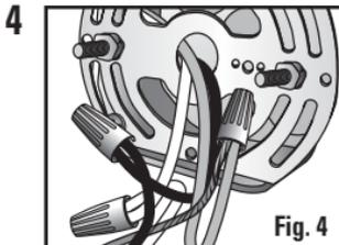
Connect the supply leads from the electrical box to the fixture wire leads using the medium wire nuts supplied in your installation hardware kit as per the illustration (Fig. 4). The black lead from the fixture goes to the black supply lead and the white lead from the fixture goes to the white supply lead.
