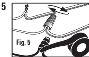
Tighten the wire nuts properly to prevent the wires from coming loose (Fig. 5). Tape the wire nuts to the wire using electrical tape. Carefully push the excess wires back inside the electrical box.
