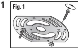
Screw the long machine screws (included) all the way into the threaded holes on the mounting bracket (Fig. 1). If your mounting bracket has more than 2 threaded holes, measure the center-to-center distance of the holes to make sure it matches the hole openings in the pan of your fixture. Screw the hex nuts onto the long machine screws until they are tight against the mounting bracket.
