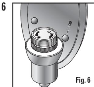
Pull any excess wire up from the fixture and through the center hole of the mounting bracket. Push the excess supply wires back into the electrical box. Move the mounting plate up to and over the mounting screws and screw on both base fasteners on opposite sides of the mounting base (Fig. 6). Hand-tighten the round fixture fasteners until the pan is securely against the wall. Make sure not to pinch any of the wires under the pan.
