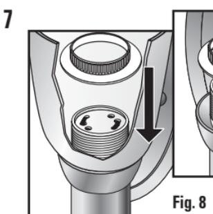
Your fixture may be packaged with the diffuser locking ring already in place. If this is the case, the diffuser locking ring will need to be removed before installing the diffuser (Fig. 7). Unscrew the diffuser locking ring by turning counterclockwise. Set aside. While holding the glass diffuser, secure the diffuser by screwing on the diffuser locking ring in a clockwise direction (Fig. 8). Hand-tighten the
