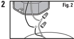
Remove the old fixture. Make yourself a sketch of how the fixture is wired (index the sketch by wire color) or mark the wires themselves with masking tape and a pencil so you will know how to connect the wires to your new fixture (Fig. 2). If several wires are involved or if the wiring seems more complicated and perhaps even includes a red wire, take note of the connections before you disconnect them.
