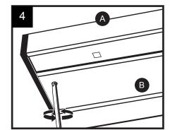
4. Once the fixture (A) is secured to the cabinet, replace the wire compartment cover (B). Plug in the power cord (C) and the installation is complete.
