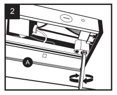
3. **KEYHOLE INSTALLATION**: Position the fixture (**A**) and mark the location of the narrow ends of the keyhole slots onto the mounting surface. Drill a 1/16 in. pilot hole into the marked screw locations. You can also use an awl or nail to dimple the screw holes. While holding the fixture in place tighten the wood screws (**AA**) with a phillips head screwdriver until the fixture is flush with the surface.
