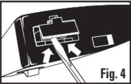
Using a flathead screwdriver, carefully pry off the plastic cap that covers the "Power-In" port on the end of the fixture (Fig. 4).
