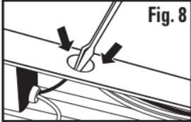
Determine which corresponding knock-out is closest to the supply wire feed and remove it (Fig. 8). **CAREFULLY REMOVE THE KNOCK-OUT BY HAMMERING A FLATHEAD SCREWDRIVER OR PUNCH UNTIL THE SURFACE BREAKS.** If the knock-out did not break free, use pliers and bend it back and forth until it snaps off.
