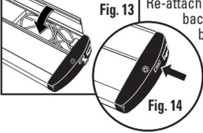
**Fig. 13** Re-attach the wire compartment cover by hinging the back edge of the cover with the channel in the back of the fixture chassis and lowering it into position (**Fig. 13**). Push both locking tabs inward to lock the wire compartment cover back into place (**Fig. 14**).
