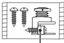
**Ⓔ NM cable strain relief connector**
