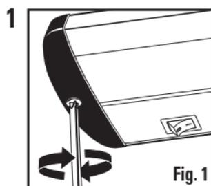
The fixture can be mounted without utilizing pilot holes. Firmly hold the fixture against the mounting surface and begin turning the mounting screws until they are fully driven in and the fixture is firmly attached to the mounting surface (**Fig. 1**). **NOTE:** DO NOT overtighten the screws, as it may result in damage to the fixture or the mounting surface. **Direct Wire Installation Only:** Determine the fixture location, but do not mount until the wiring steps are completed.
