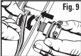
Attach the supplied strain relief by inserting the threaded end (from outside the fixture) through the knock-out. Secure the strain relief to the fixture's chassis by tightening the fastener (from inside the fixture) (Fig. 9). **NOTE:** Remember to have the strain relief screws oriented in a manner that allows tightening/loosening of the clamp screws after the fixture has been attached to the mounting surface.
