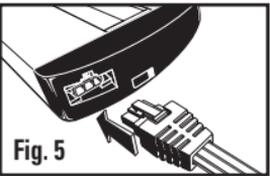
**WARNING: DO NOT plug the power cord into the power supply before completing the installation.** The power cord has a grounded plug at one end and a connector plug at the other end. **FIRST:** Insert the connector plug into the power port located near the on/off switch at the end of the fixture (Fig. 5). The cord connector plug will
