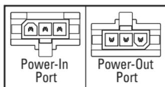
Before mounting, find a suitable location to mount the fixture that will reach the power supply (within 5 feet) or to reach adjoining fixture (within 18 inches). The fixture has two power ports located at each end of the fixture. The "Power-In" port is located on the end next to the on/off switch and is used to connect the fixture to a power supply. The "Power-Out" port is located at the opposite end and is used to link power to additional fixtures connected together.
