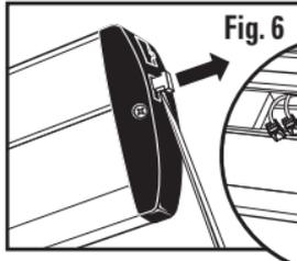
Located on each side of the fixture are two tabs that lock the cover to the wire compartment in place. Disengage each tab by carefully pulling them out with a flathead screwdriver (Fig. 6) far enough to remove the cover to expose the wire connections and keyhole slots inside (Fig. 7). **DO NOT** try to remove tabs from the fixture.
