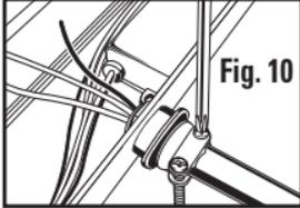
Insert the flexible whip or NM cable through the strain relief and tighten the clamp until it is secure (Fig. 10). Allow enough wire length to make the connection.
