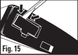
**Fig. 15** Using a flathead screwdriver, carefully pry off the plastic cover that protects the "Power-In" port on the the fixture being added (**Fig. 15**). Carefully pry off the plastic cover that protects the "Power-Out" port on the the fixture it is being linked to.
