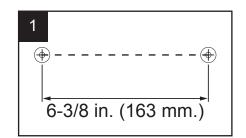
2. Use a nail or awl to dimple the surface to help guide the screws. Either drive the wood screws (**AA**) directly into the surface or drill two 1/16 in. pilot holes to make installing the screws easier. The screws must be driven in straight. Tighten until 3/8 in. of the screws is protruding below the surface.
