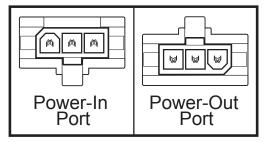
Before mounting, find a suitable location to mount the fixture that will reach the power supply (within 5 feet) or to reach adjoining fixture (within 18 inches). The fixture has two power ports located at each end of the fixture. The "Power-In" port is located on the end next to the on/off switch and is used to connect the fixture to a power supply. The "Power-Out" port is located at the opposite end and is used to link power to additional fixtures connected together.
