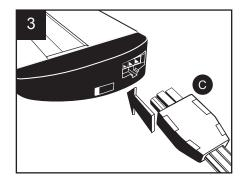
Insert the opposite end of the linking cord into the "Power-In" port of the additional unit. NOTE: Each light can be individually operated by the on/off switch located on each fixture.
