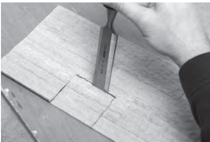
Cutting the inside edge with chisel
