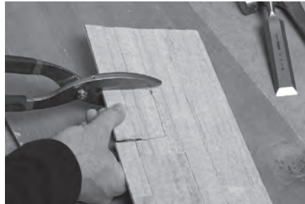
Starting a notch using a snip
